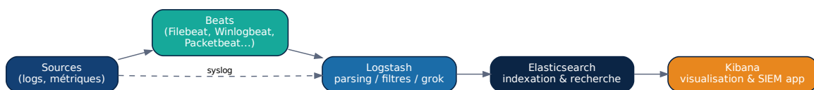
Figure 2.3: Stack Elastic : Beats/Logstash → Elasticsearch → Kibana (application SIEM).
